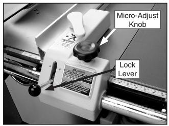
Figure 56. Rip fence micro-adjusting controls.
